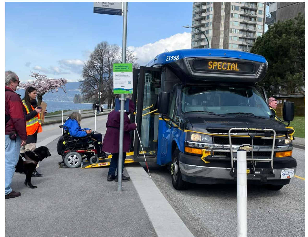
Figure 8: Wheelchair Ramp Deployed onto Island Platform Bus Stop, Vancouver, British Columbia
