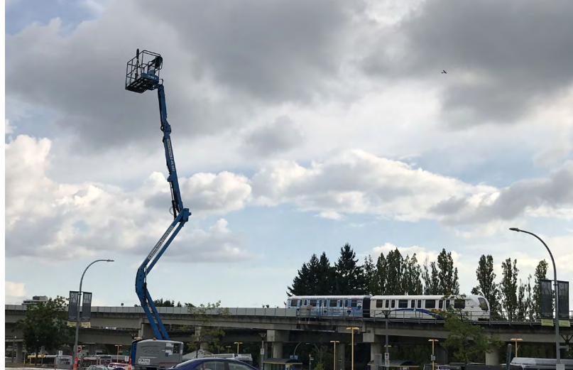
▲ SkyTrain noise measurements should be taken well above the guideway (Photo: BKL)
