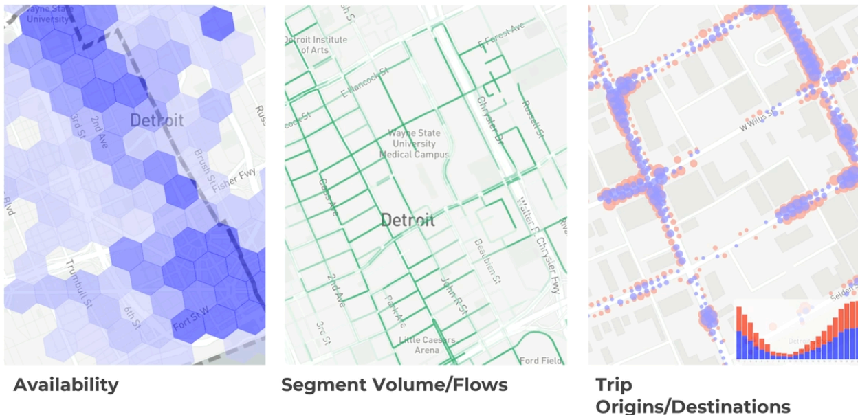
Figure 5 The same MDS data produces three distinct visualization analyses, all of which may be useful for different planning purposes. Source: SharedStreets (2019)
