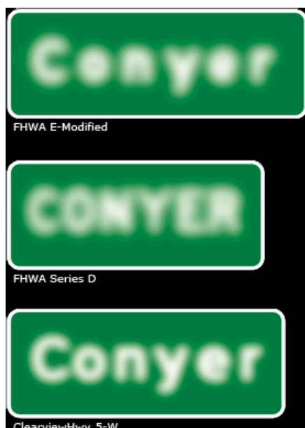
Clearview Hwy (bottom) is more legible than standard FHWA typefaces under halation testing which simulates impaired vision.
