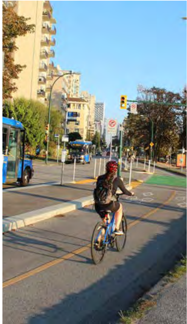
Figure 30 – Quick build floating bus stop Beach Avenue, Vancouver
