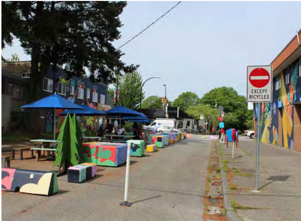
Figure 44 – Concrete barriers, flex post, and signage used to divert motor vehicle traffic along W 17th St, Vancouver
