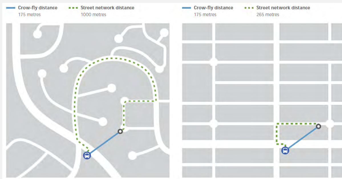
Figure 3 - Walking distances are shorter in more connected networks (source: TransLink Transit-Oriented Communities Primer).
