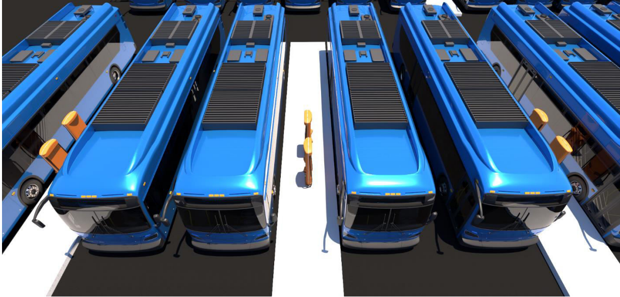
Figure C-8 Depot Charging with ground-mounted CCS corded chargers
