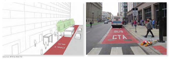
Figure C7.2: Diagram (Left) and Example of Offset Bus Lane, New York MTA Select Bus Service (Right)
