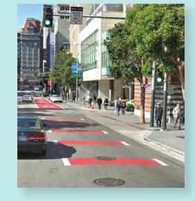
• The United States Federal Highway Administration has found that by adding right turn lanes at major intersections, collisions between right turning traffic and through traffic can be reduced by 5%. By using part of a transit lane to lengthen the deceleration area for right turning traffic, all collisions can be reduced by an additional 10%.<sup>2</sup>
