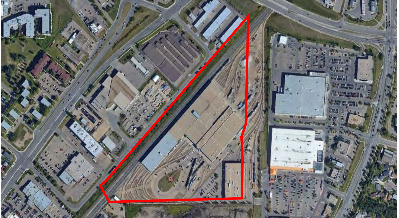
Figure 7-3: D.L. MacDonald Yard, Edmonton. Approximately 9 hectares with 1,560 linear metres of storage track. Stores 60 x 26m LRT vehicles. Turnaround tracks occupy large portions of the site.
