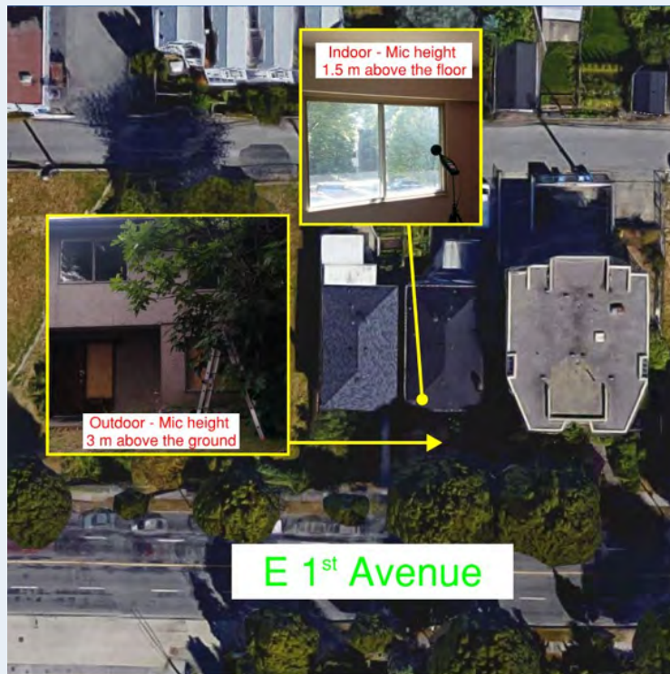
Figure C.1: Example Measurement Locations, Site 1
