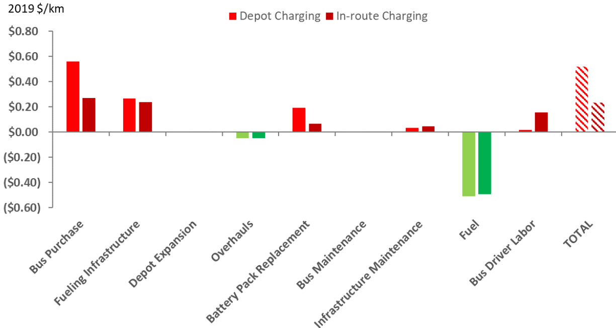
Figure D-2 Incremental Cost of MY2019 Electric Buses versus Diesel Buses (2019 $/km)
