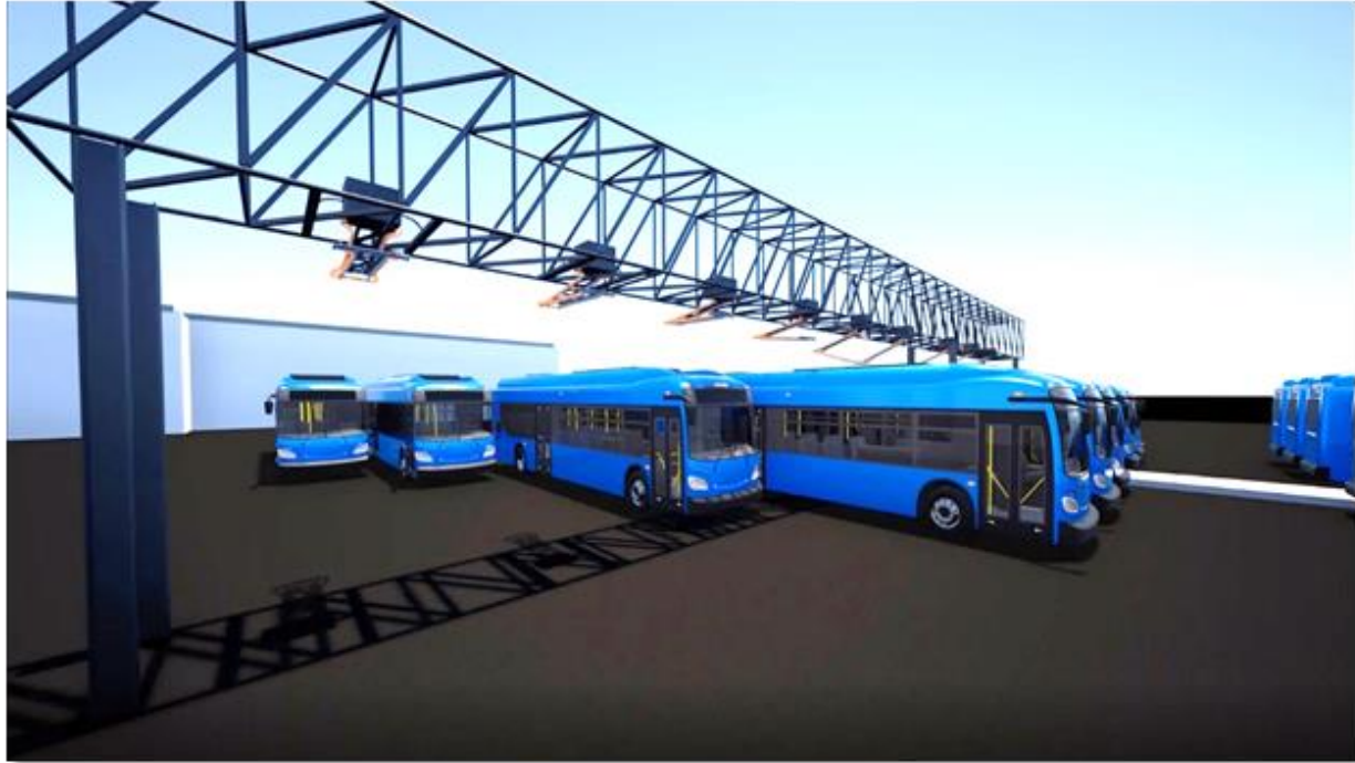
Figure C-10 Depot Charging with SAE J3105-1 conductive pantograph chargers
