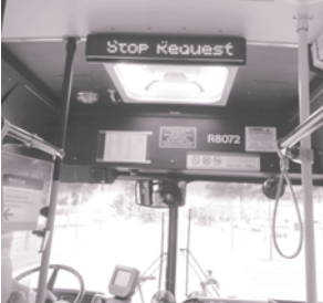
Ceiling-mounted electronic displays will soon display information about the next stop on a bus route.
