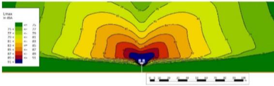
**Scenario #2** – This figure represents an intermediate rail surface condition and noise level and is 5 dB quieter than Scenario #1. In areas of the SkyTrain system where harder rail steel is already in use, this is a common scenario.
