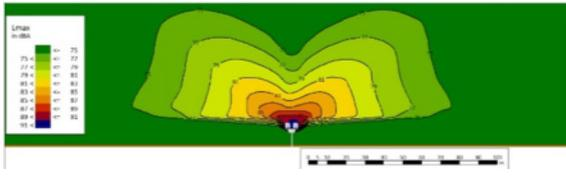
**Scenario #3** – This figure represents a good rail surface condition and is 10 dB quieter than Scenario #1. This noise level is common around the network after grinding takes place.
