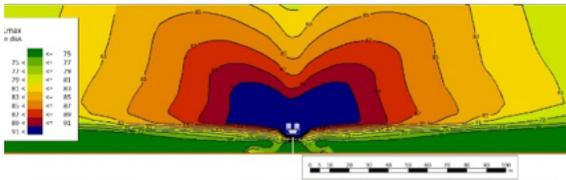
**Scenario #1** – This figure shows what the noisiest areas (mostly on the original Expo Line) are currently like in times when the rail surface condition is at its worst before grinding.
