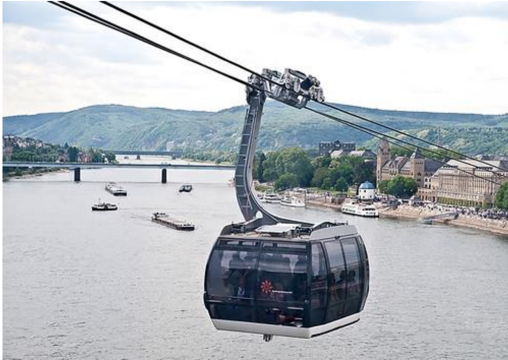
Figure 2.2 Example of a 3S Ropeway Tri-cable System on an Urban Gondola. The Koblenz Rheinseilbahn located in Koblenz, Germany
