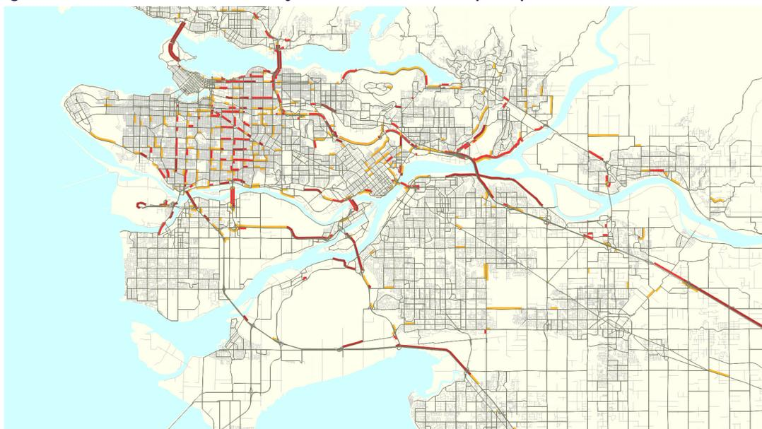
Note: Congestion is defined as aggregate vehicle hours of delay on each link experienced in the AM peak hour, where vehicle delay is calculated as hours of delay over and above the LOS D performance level multiplied by the vehicle volume (Legend: Orange: 10-30 hours; Red: 30-60 hours; Maroon: >60 hours).
