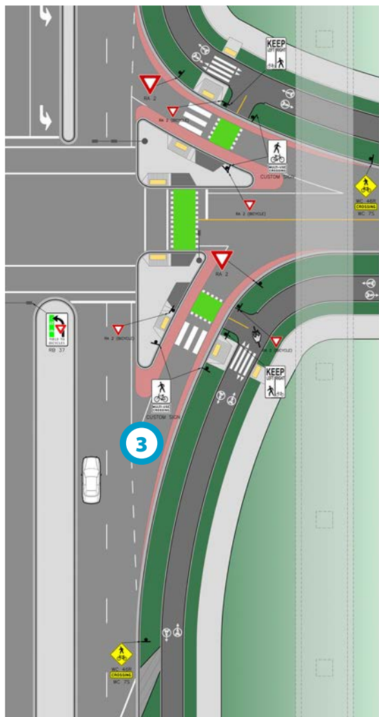
FIGURE 15 - CHANNELIZED INTERSECTION WITH SEPARATED CROSSINGS
