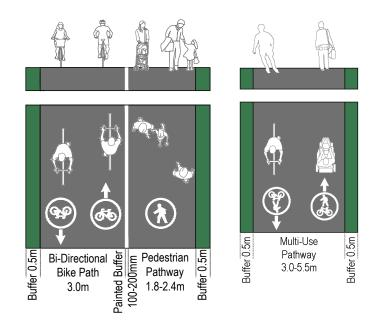
FIGURE 10 - CONSTRAINED PATHWAY WITH PAINT SEPARATION (LEFT) FIGURE 11 - MULTI-USE PATHWAY (RIGHT)
