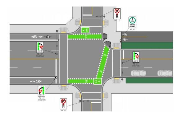
FIGURE 38 - TRANSITION MULTI-USE PATHWAY TO ON-STREET (AND VICE VERSA) BI-DIRECTIONAL TO UNI-DIRECTIONAL - EXAMPLE 2
