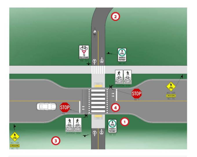
FIGURE 33 - MID-BLOCK UNSIGNALIZED MULTI-USE CROSSING - CURB EXTENSION
