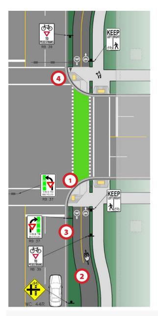
FIGURE 19 - BEND-IN SEPARATED CROSSINGS
