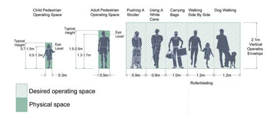
FIGURE 3 - TYPICAL DIMENSIONS FOR PEDESTRIANS (SOURCE: ADAPTED FROM THE B.C. ACTIVE TRANSPORTATION DESIGN GUIDE)
