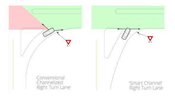
FIGURE 24 - CONVENTIONAL VERSUS SMART CHANNELIZED RIGHT TURN LANES
