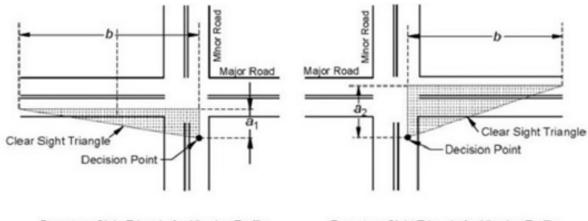
Departure Sight Triangle for Viewing Traffic Approaching the Minor Road from the Left Departure Sight Triangle for Viewing Traffic Approaching the Minor Road from the Right
