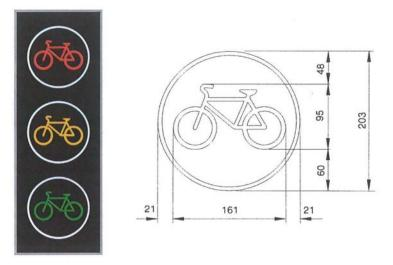
FIGURE 41 - BICYCLE TRAFFIC SIGNAL HEAD DISPLAY
