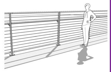
the sense of obstruction and enclosure. Given the length of the site, railings should be easy to install, repair, and replace. Railings should also be as transparent as possible to maximize the openness of the site. The design of handrail and guard for landscaping should follow design standards found in Section 3 of the *Design Principles & Standards manual and the Building Code*. Handrails and guards should be:
