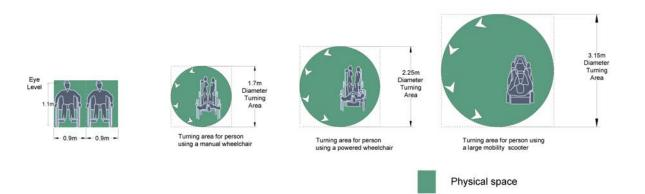
FIGURE 4 - TYPICAL WHEELCHAIR OPERATING SPACE (SOURCE: ADAPTED FROM B.C. ACTIVE TRANSPORTATION DESIGN GUIDE) 20
