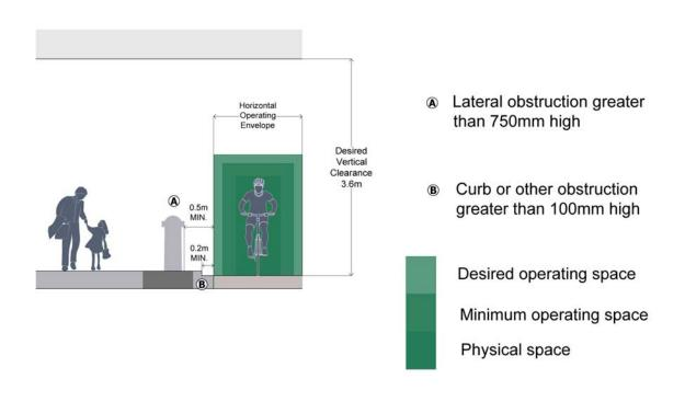
FIGURE 7 - MINIMUM HORIZONTAL AND VERTICAL CLEARANCES (SOURCE: ADAPTED FROM B.C. ACTIVE TRANSPORTATION DESIGN GUIDE)
