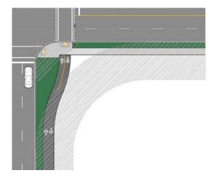
FIGURE 23 - RECONFIGURED CHANNELIZED INTERSECTION High entry angle approaches also make pedestrians and bicycle users more visible at the crossing. **Figure 24** illustrates the difference between conventional channelized right turn lanes compared to a 'smart channel' right turn lane.
