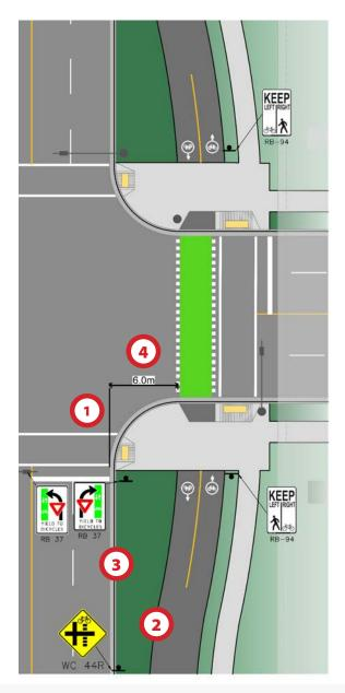
FIGURE 21 - BEND-OUT SEPARATED CROSSINGS
