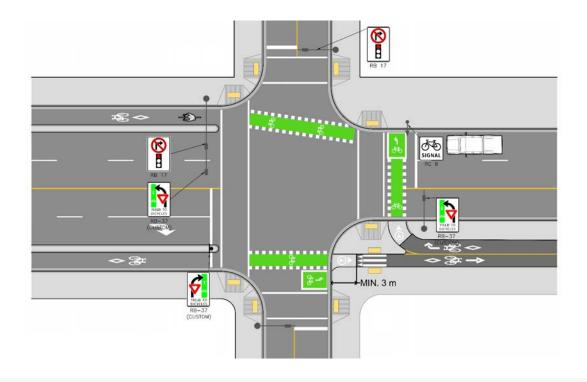
FIGURE 37 - TRANSITION SEPARATED PATHWAY TO ON-STREET (AND VICE VERSA) BI-DIRECTIONAL TO UNI-DIRECTIONAL - EXAMPLE 1
