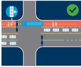
Active signal priority includes detecting an approaching bus in advance of an intersection and extending green times so the bus doesn't wait at the signal.
