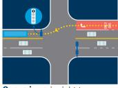
Queue jump in right-turn lane or BAT lane without a receiving lane. A specialized transit signal and / or phase is required to help the bus transition back into traffic.
