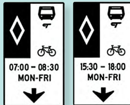
Figure C6.4: Peak-Hour Sign on Traffic Light in Calgary<sup>4</sup>
